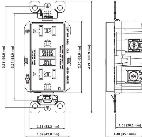
20A SmartlockPro® Self-Test GFCI
