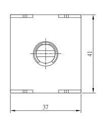
DUTY=10% STROKE=2mm FORCE=2930gf DUTY=10% STROKE=10mm FORCE=1680gf MAX 0N TIME =2sec
